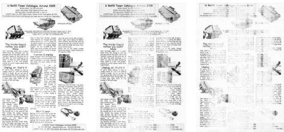
As you can see, the faded area gets wider and more pronounced with each print, but even on the last very faded page, the print at the edges is still the same blackness as on the first print. If you take out the cartridge and give it a shake at this point, perfect print will return for a few more prints – but then the fade out will return again. This pattern of progressively widening fade out bands which can be temporarily cured by shaking is the hallmark of toner exhaustion.
